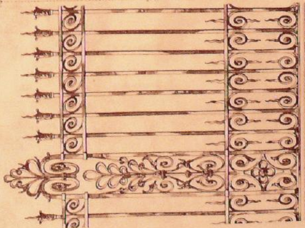
Main Standard with Backstay repeats every 10' 6", and is included in the price of the railing.
