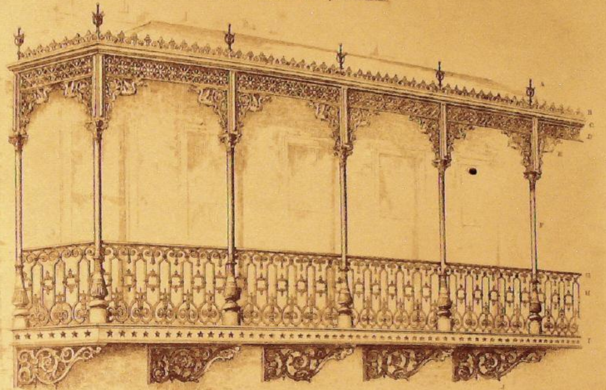
A No. 181 TERMINAL 1'6". B No. 82 CRESTING 7". C No. 45 QUETER 6" x 4". D No. 109 FRISK RAIL 1 1/2". E No. 68 BRACKET 1'6" x 1'6". F No. 121 COLUMN WITH BRACKET BRASS. G No. 5 HANDRAIL 1 1/2" x 1 1/2". H No. 606 BALUSTIN RAILING 2' 10". I No. 3 PERFORATED GUARD. J No. 17 BRACKET 2' 11" x 1' 6". ORNAMENTAL FLOOR PLATE SOLID OR PERFORATED, 6" x 6"
