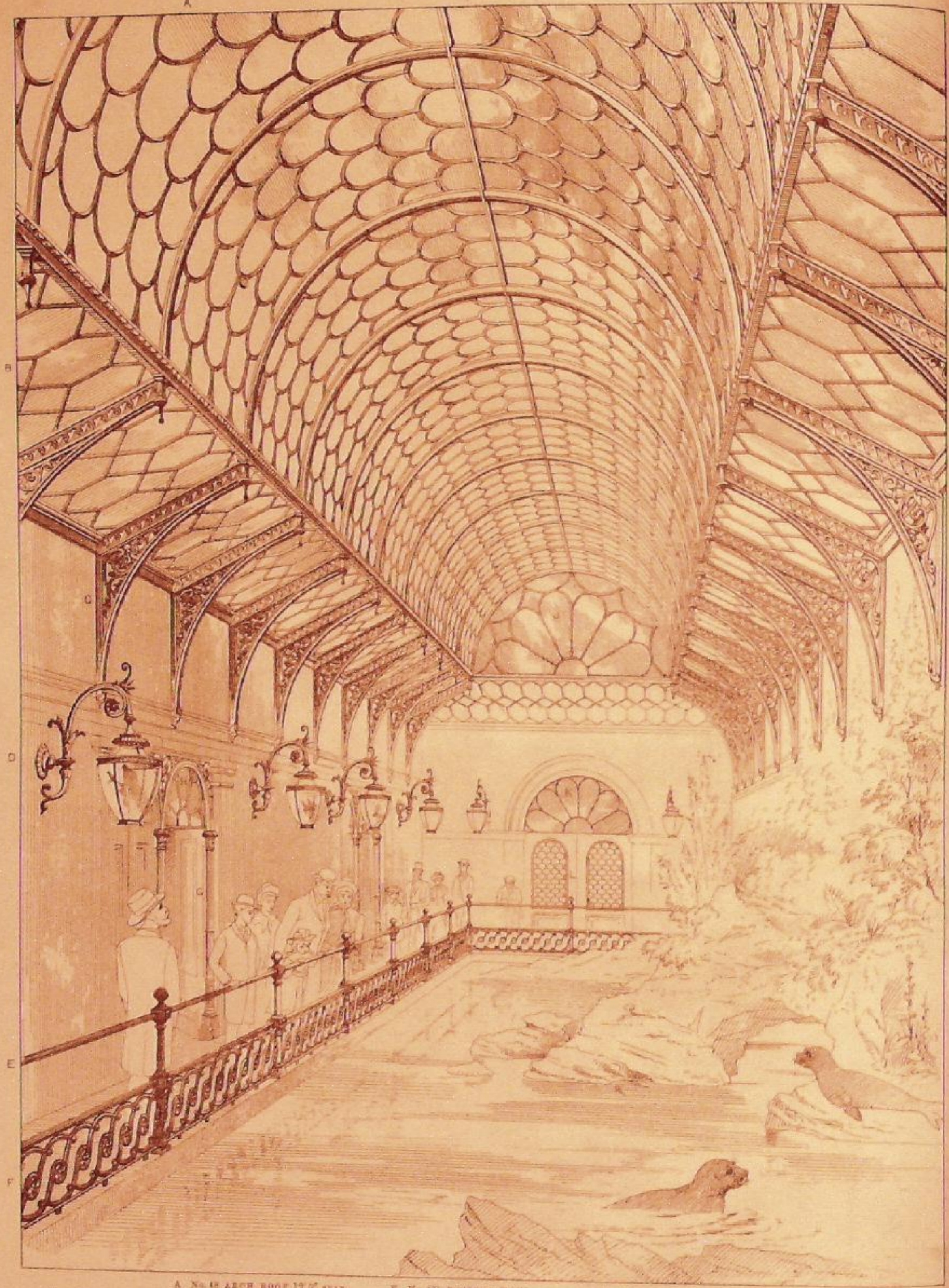
A No. 18 ARCH ROOF 17' 6" span. B No. 12 WINDOW C No. 61 ROOF SPANDRIL D No. 72 LAFF BRACKET E No. 471 RAILING 7' 10" F No. 1119 RAILING 7' 10" G No. 115 COLUMN C. H No. 32 FANLIGHT WINDOW I No. 10 SPANDRIL ARCHES J No. 24 SEMICIRCULAR WINDOW K No. 35 SEMICIRCULAR WINDOW L No. 29 WINDOWS
